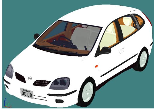
Fig. 1. Geometry of a production car model. This surface data is based on a CAD system and consists of over 15 million polygons.
