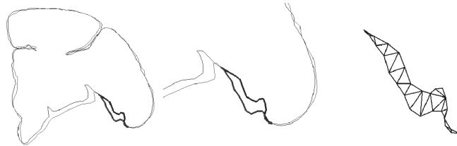
Fig. 3: “Ribbon” surface reconstruction . From the left: a pair of adjacent sections; detail of a region delimited by two points of intersection; detail of the region triangulation.
