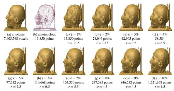
**Figure 4:** Comparing the visualization of the CT head dataset rendered as a conventional volume object and as a PBVO. Several point clouds were extracted from the original dataset with different numbers of points (voxels).
