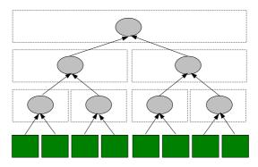
**Figure 2:** A binary tree representation. The squares represent the original data-points, and the ellipse nodes contain a basis function and the corresponding coefficient. The dashed box around the node indicates the width of the support of the function.
