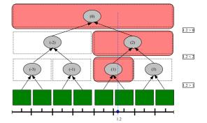
Figure 5: Traversal of a basis node tree, reconstructing the value at position 1.2. The method starts at the root node, and checks in which child the coordinate lies. Nodes traveled through are highlighted.
