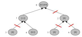
Figure 3: Pruning the nodes from the bottom up in a binary space partitioning tree. Starting with node 6, we can remove it because its coefficient is zero. Node 5 can be removed for the same reason, and node 2 now becomes a leaf. This node can be removed as it is 0. Node 4 is saved and node 3 is removed, but then the pruning stops since there are no more leaves to check.
