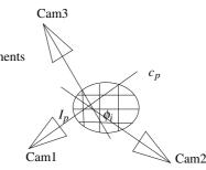
**Figure 1:** The reconstruction process: The coefficients of the basis functions  $\phi_i$  are restricted by several camera views.  $I_p$  is the image intensity and  $c_p$  the backprojected ray of pixel p.
