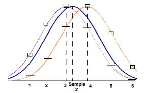
Figure 6: Illustration of the ACCC method with two grid point kernels: The kernel for any sample point between grid point 3 and 4 is within the narrow band of the kernels on grid point of 3 and 4.
