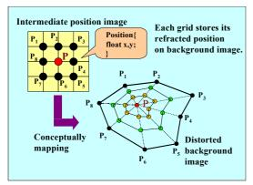
Figure 7: Post-refraction super-sampling
