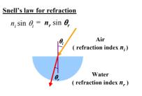
Figure 1: Snell's law for refraction.
