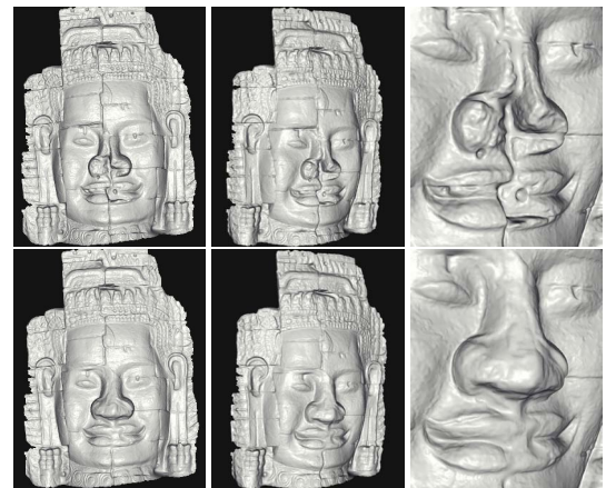
Figure 11: One experimental result of our proposed restoration method, face No. 49E, with comparison from a side view and enlarged partial details. Upper: measured shape. Bottom: restored output.
