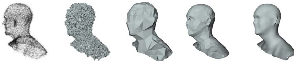
Figure 6: Comparison to other reconstruction algorithms. From left to right: Initial point cloud with 1 percent gaussian noise; reconstruction using Powercrust [ACK01], Robust Cocone [DG04], QPoly [OBS05] and our method.
