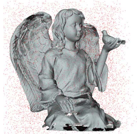
Figure 1: Surface mesh and outliers, reconstructed from a point cloud with 2,008,414 points and 10K random outliers. Data set courtesy of the U.C. Berkeley CAM Group.
