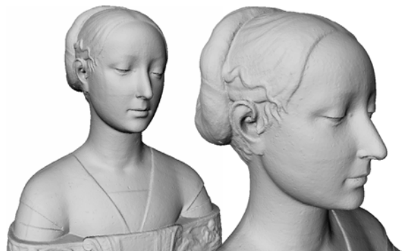
Figure 1: Sforza . Our variational method allows high-fidelity reconstruction of unprocessed point sets (3D scanned Sforza, 200K points). The final mesh is extracted via isocontouring of a scalar function computed through optimization.
