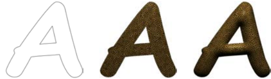
Figure 2: Repoussé workflow: the flat domain bounded by the input curves is triangulated and the resulting surface is inflated.
