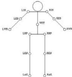
Figure 2: The stick figure model containing 13 joints (labelled by their abbreviations) and 12 bone segments.
