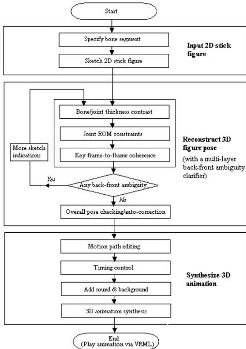
Figure 1: Overview of system working pipeline.
