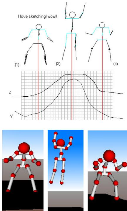
**Figure 9:** Motion definition:  $Y$  and  $Z$  curves specify a motion, and the drawing speed of  $Y$  curve indicates motion timing.
