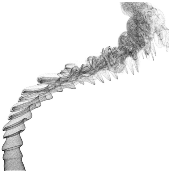
Figure 8: Control of large scale flow features. The image shows the evolution of a jet, guided along a spiral curve using a discretized vortex tube.
