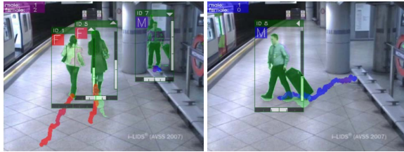
Figure 3: Screenshots of our full-body based real-time visual traits classification: no high resolution faces available, varied postures, illumination and occlusion.
