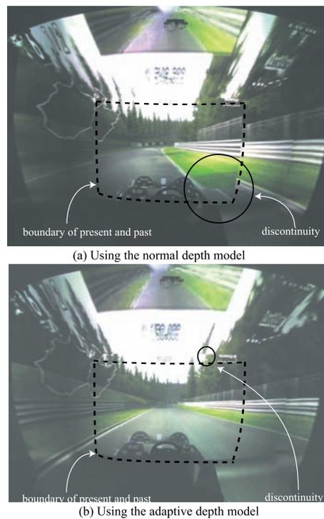
**Figure 5:** Effect of adaptive depth model
