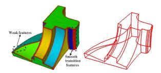
**Figure 1:** Multi-type feature classification on the Fandisk with Gaussian noise ( $\sigma = 5\%$  of mean edge length). Patch features are shown in different colors, while curve and point features are colored in red. Our method can detect weak features and smooth transition features (left). The connected curve features are highlighted as a wire-frame representation (right).
