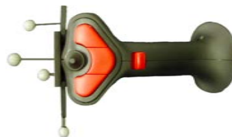
Figure 3: The flystick used for interaction has several buttons for triggering interactions and reflecting markers for tracking with IR cameras.
