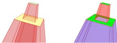
Figure 2: In traditional shadow volumes, shown on the left, all polygons are quadrangles with two affine and two ideal ( w=0 ) vertices. By contrast in the set union of the shadow volumes, shown on the right, some polygons are defined by four affine vertices.
