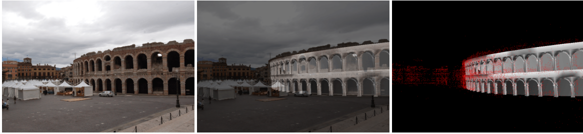
Figure 4: Example of mixed reality overlay from a localized view. On the left the original image; in the middle a superimposed 3D model of the Arena; on the right the 3D model with the points cloud in red.
