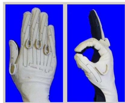
**Figure 4:** The positions of the hand used by the calibration software provided with the CyberGlove software.
