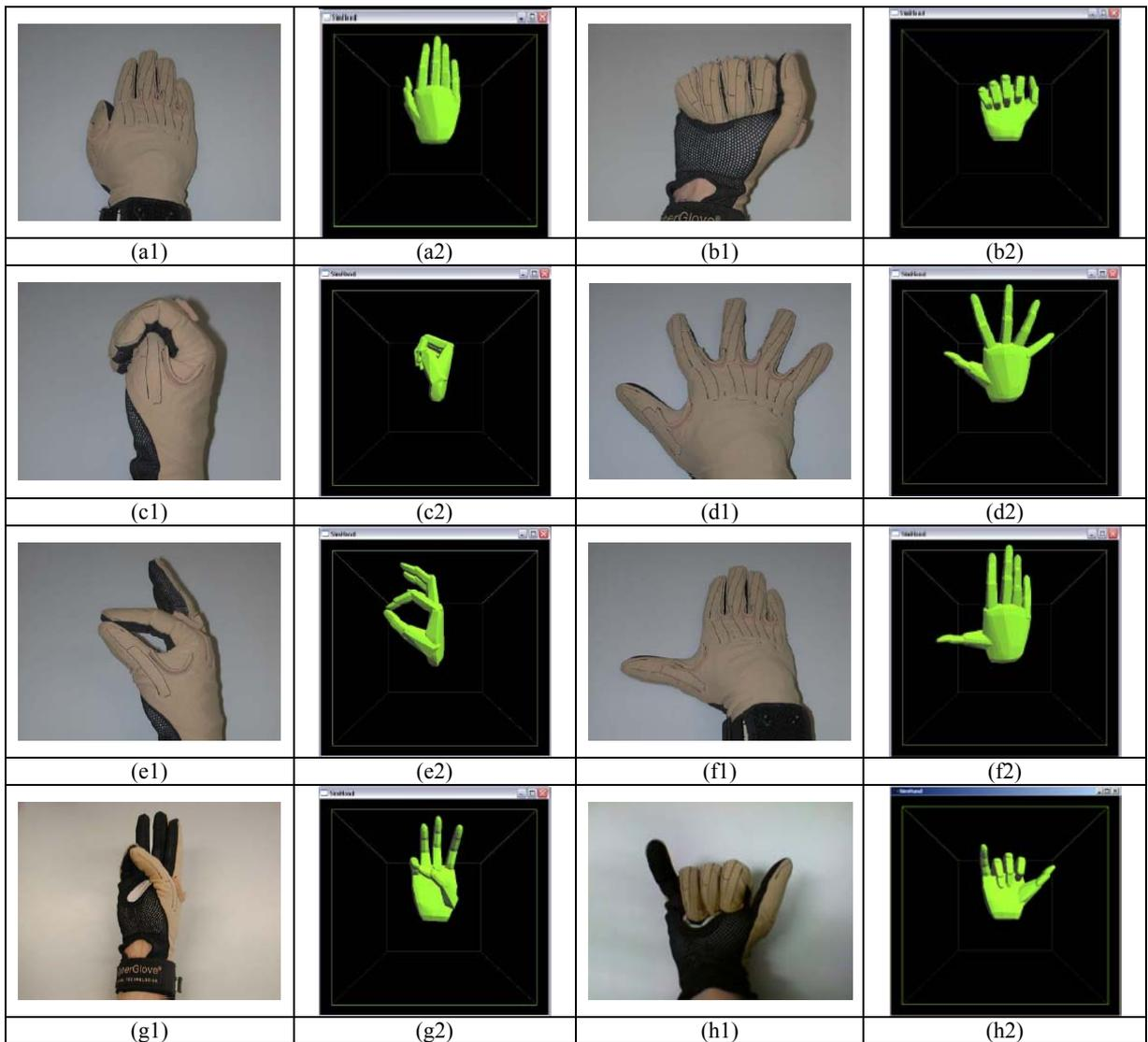
**Figure 7:** Photographs report the seven poses assumed by the user hand during the glove calibration step. The images represent the rendering of the virtual hand.
