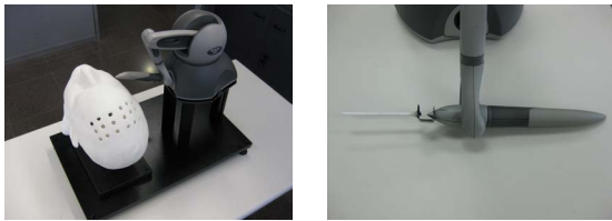
Figure 1: In the left image, the general aspect of the prototype without the screen is shown. In the right image, the plastic tube which simulates the catheter is presented.
