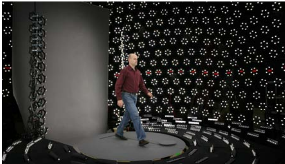
Figure 1: The treadmill, turntable, and lighting apparatus used for capturing human locomotion from multiple viewpoints under time-multiplexed lighting. Behind the person is the background matte; the vertical array of high-speed cameras is out of frame to the right.
