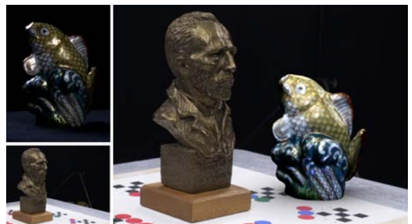
Figure 1: By analyzing multi-view images of the fish, and the Van Gogh statue, captured under a fixed unknown illumination (left), we are able to extract the diffuse/specular texture of these objects as well as the environmental illumination map. These results help us perform advanced scene manipulations such as inserting the fish into the Van Gogh scene (right).
