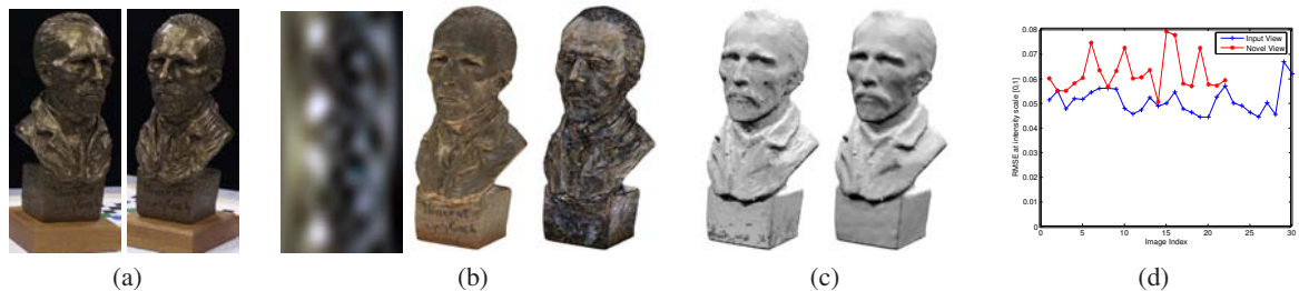
Figure 12: (a) Two of the 30 input images of the Van Gogh data set. (b) Estimated illumination, diffuse albedo, and specular albedo. (c) Estimated specular bump map compared with the original surface shape (right). (d) RMSE of the synthesized images in all 30 input views, (blue line, average RMSE = 0.0507) and 22 novel views (red line, average RMSE = 0.0619).
