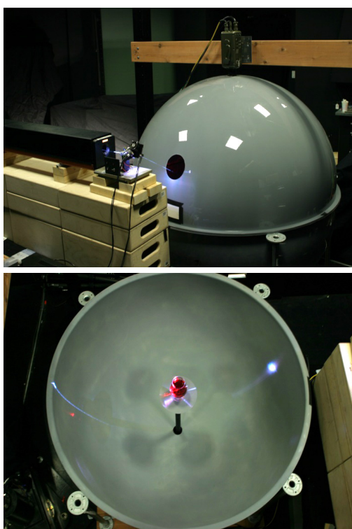
Figure 2: (a) A dual light stage comprises a sphere, a laser, a 2-axis galvanometer scanner, and a video camera. (b) The top half of the sphere has been removed to show the object inside. We can see the patterns of reflected light on the inside of the sphere.
