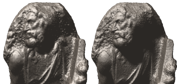
Figure 1: Images of the St. Matthew statue (372M triangles) rendered with state-of-the-art polygon based out-of-core rendering (left) and with our algorithm including soft shadows (right). Notice how the left picture appears blurred due to the lack of fine details.
