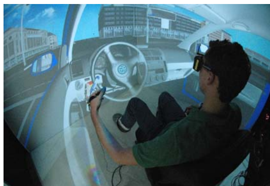
Figure 1: A user interacting with a virtual car interior in a projection-based immersive environment
