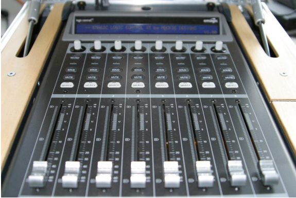
Figure 2: A MIDI mixer with motor faders for hands on control of node properties.
