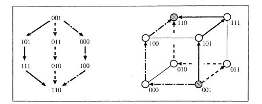
Figure 3: Hypercube message routing
