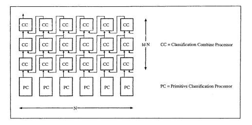
Figure 4: Block Diagram of Raycasting Machine [23]
