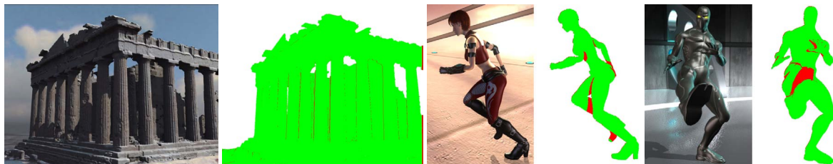
Figure 1: Real-time rendering applications exhibit a considerable amount of spatio-temporal coherence. This is true for camera motion, as in the Parthenon sequence (left), as well as animated scenes such as the Heroine (middle) and Ninja (right) sequences. Diagrams to the right of each rendering show disoccluded points in red, in contrast to points that were visible in the previous frame, which are shown in green (i.e., green points are available for reuse). [Images courtesy of Advanced Micro Devices, Inc.]
