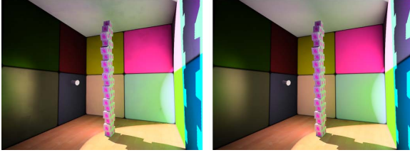
Figure 25: Imperfect shadow maps still show some artifacts with 256 VPLS, which can be smoothed out using TC. Image courtesy of Martin Knecht.
