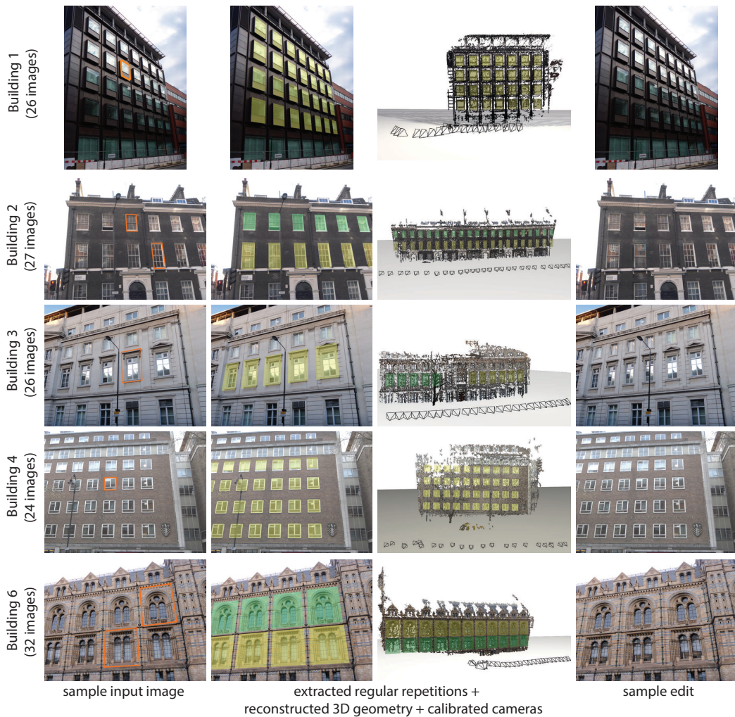
Figure 4.7: For each example, we provide a sample input image, the user marked template in a single image (orange), the extracted repetition pattern and the calibrated cameras. This information is used for a range of image manipulations.
