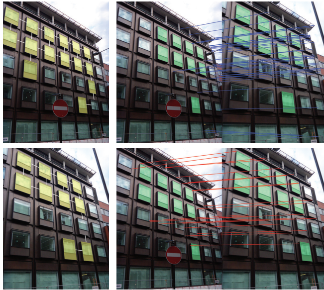
Figure 4.3: Given a pair of images with their detected grids (left), for each candidate alignment we detect the overlapping grid regions (shown in green). We compute feature matches outside the overlapping regions and count the number of matches supporting the candidate alignment. Top-right shows the correct alignment with highest support (51 matches) and the bottom-right is a wrong candidate alignment (25 supporting matches).
