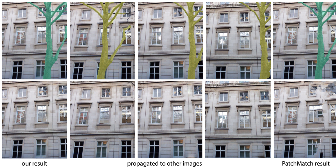
Figure 4.12: Occlusion mask marked in one image (top-left) is propagated to the other images. Occlusion removal using propagated information from other images provides significantly improved results compared to the single-image based state-of-the-art PatchMatch [8] method.
