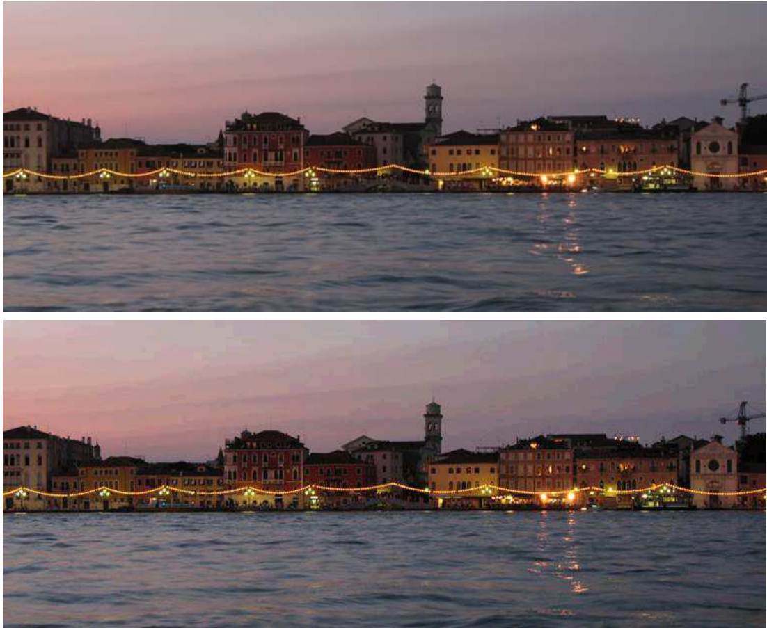
Figure 1.7: An example of quantisation errors during visualisation of LDR content on HDR monitors: On the top a LDR image of Venice bay. On the bottom a simulation of the same image on an HDR monitor. Linear stretching produces artefacts in the form of contouring.
