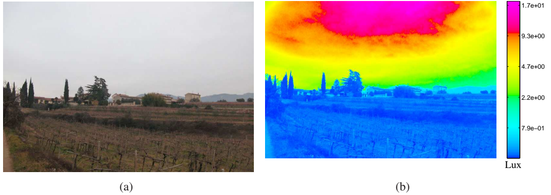
Figure 5.4: An example of expansion for well-exposed content for the Vineyard LDR image: a) The original LDR image. b) The false colour image of the expanded image in a) using Equation 5.7 with L_w, \text{Max} = 20 and L_w, \text{white} = 40 . Note that there are no over/under-exposed, so there are no missing areas with details and colours.
