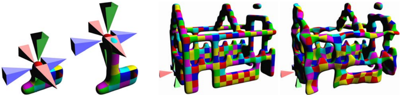
Figure 1.16: Simple Lego-style modeling with subdivision surfaces. The cursor with \pm x/\pm y/\pm z arrows can be moved back and forth with pairs of neighbouring keys q,w/a,s/z,x . Swift control is surprisingly fast and easy to learn for users with a good spatial imagination. Jittering the control vertices yields a nice rubber-like appearance.
