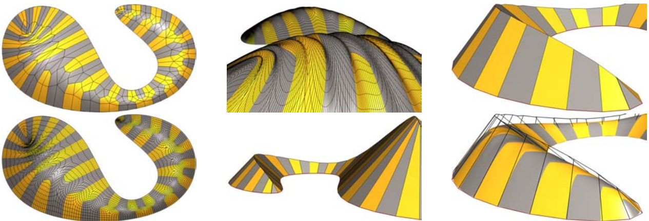
Figure 4.74: Subdivision surface from irregular straight skeleton. The small edges in the center of the left end lead to surface wobbling (1a, 1b, 2a), an effect that is explained in Fig. 4.69. The surface on the thin end is not completely smooth either because of the varying surface degrees. Also note that the spine curve contains several slight hills (1c,2c). The reason is that more bisector rays from the outer than from the inner part of the polygon boundary arrive at the spine. So the rays from the outer boundary are slightly longer, i.e., they reach higher.
