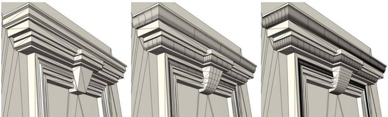
Figure 4.30: Combined B-rep example: Levels of window detail. Architectural models typically exhibit rounded features only in few, but very distinct places. Efficient LOD control is vital for interactive inspection of interesting building details (c). But when the user just passes by a house with many windows, a low LOD is needed (a).
