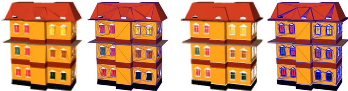
Figure 4.12: Adaptive level of detail with progressive meshes. The low resolution has only 14%, or 558 from 3992 vertices. At a low pixel resolution (a,c), the difference is hardly noticeable, despite the distortion of (b).
