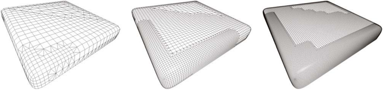
Figure 3.39: Adaptive display of subdivision surfaces.
