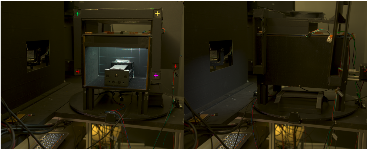
Figure 4.7: The front and side view of the real-scene box and schematic of the calibration target inside. The calibration target has a grid of four-by-six squares of the size 30 mm x 30 mm, which defines a world coordinate system. The red, green, and blue arrows in the figure represent the origin and orientations of the X, Y, and Z axes, respectively. We define the upper-left corner of the grid as the origin for the X and Y axes and the target placed at the front location as the Z = 0 plane.
