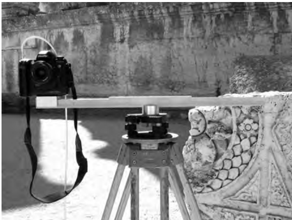
Figure 1: Using just one digital SLR camera on a calibrated base bar.
