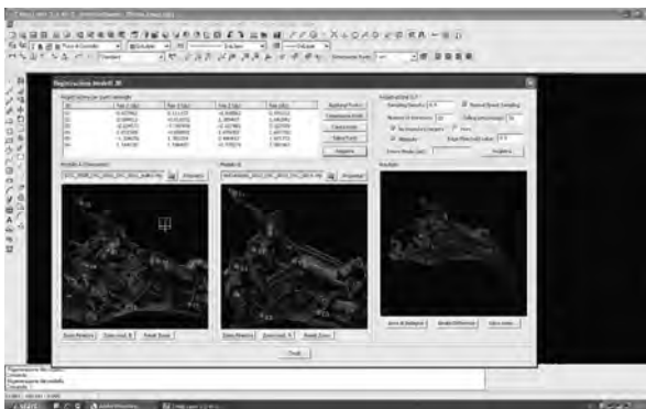
Figure 5: Registration of two different point clouds using Z-Map Laser Software
