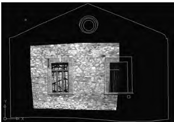
Figure 6: The rectified image with the rectification software overlaid with the vector restitution of the object
