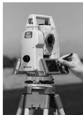
Figure 1: The Topcon GPT 7000i Imaging total station
