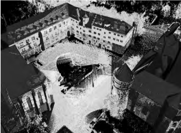
Figure 4 : Point cloud from StreetMapper aligned with available 3D city model.
