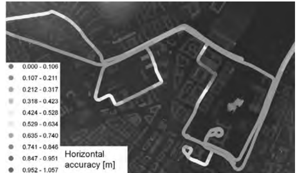
Figure 6 : Estimated horizontal accuracy of the trajectory after GNSS/IMU post processing.
