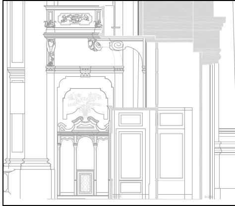
Figure 9: Extract of a section with decorative elements recovered from rectified images
