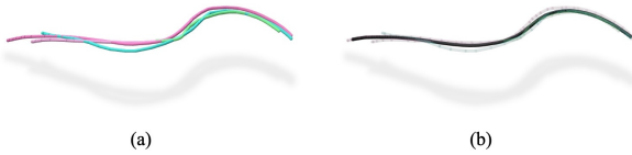
Figure 7: Consolidation results. (a) Shows multiple over-sketches, each rendered using a random color assigned to it. (b) The consolidated curve overlaid on the original strokes with reduced transparency.
