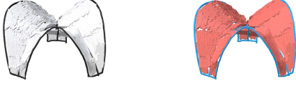
Figure 5: Left: the original sketch of a pavilion with three legs. Right: the classifier's predictions on strokes with Shape Strokes colored in blue and Scribble strokes in red.
