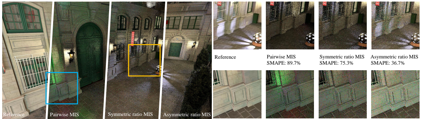
Figure 10: In the BISTRO scene, when using a large number of temporal samples M = 1000 and disabling the boiling filter. Bitterli et al. [BWP*20] introduce several artifacts like "boiling" on the ground and walls. This results in some regions appearing overly bright due to spatial reuse, while the overall image appears darker. In the "BPW" approach, we utilize the ray-traced bias correction mode for temporal reuse and pairwise MIS for spatial reuse. In both "DPW" and "ADPW", we employ symmetric ratio pairwise weight or asymmetric ratio pairwise weight for temporal and spatial reuse, respectively. Our method effectively suppress the boiling effect and reduce bias, particularly in ADPW.
