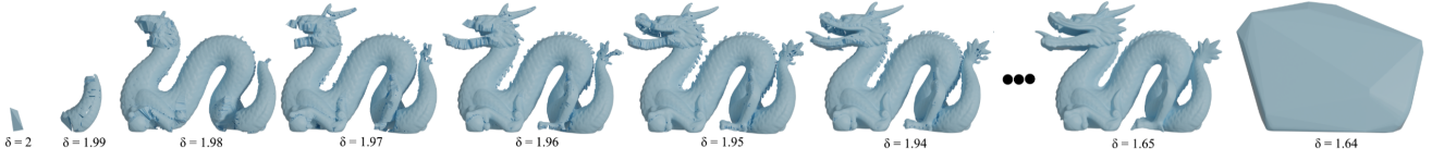
Figure 5: Automatic parameter tuning procedure: Starting from a seed tetrahedron ( \delta = 2 ), we iteratively decrease the \delta threshold value until there is a sudden decrease in the vertex count of G(\delta) (here, \delta=1.64 ) and returns the G(\delta) from the previous iteration (here, \delta=1.65 ).
